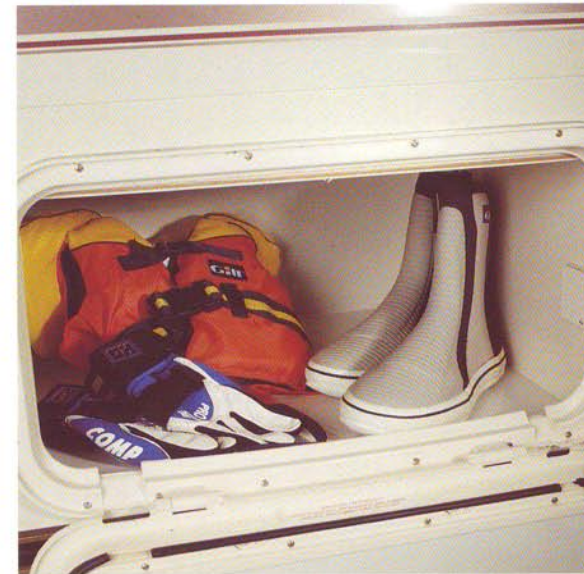
The exterior access wet locker with mains socket on the Spectrum
